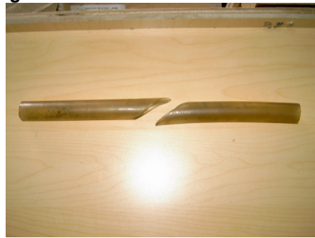
Figure 3b: Severed Untreated Tubing
